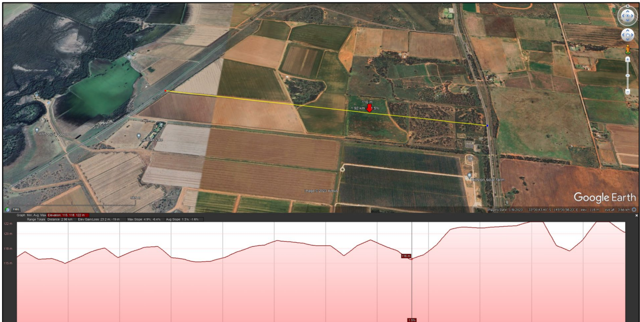
Figure 3-26 East/West elevation profile from Kidman Way through the development site to Lachlan Valley Way (Source Google Earthpro, 2023)
